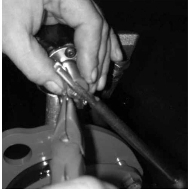
20. Fit the slotted end of the handle into the lower pivot, position the handle so that the hole in the handle lines up with the pivot hole. Carefully insert the pivot pin.
