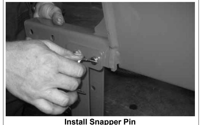
**Fig. 7 FRAME AND LEG ASSEMBLY**
