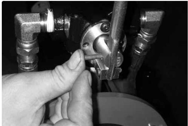
21. Using needle nose pliers, secure the pivot pin by re-inserting the cotter pin. Test the function of the handle to ensure everything is assembled properly.
