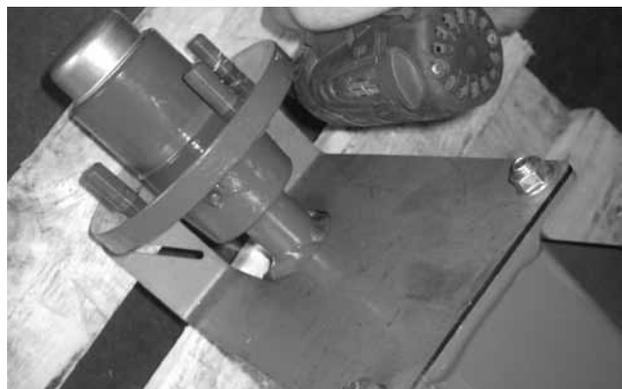
**Remove Fasteners from Axle Shipping Brackets**
